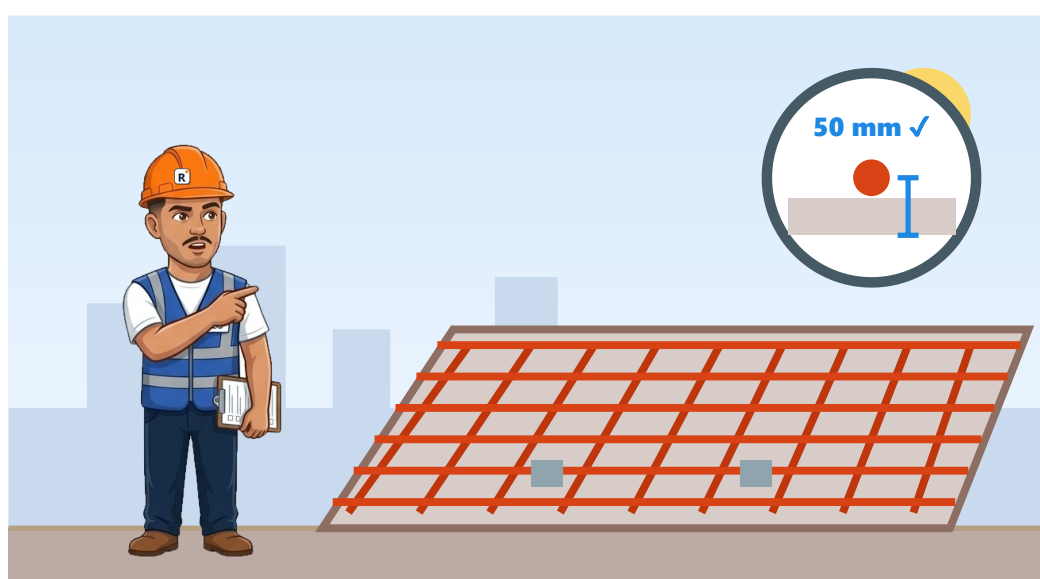
Slab reinforcement with spacer blocks and chairs, tape measure showing cover
